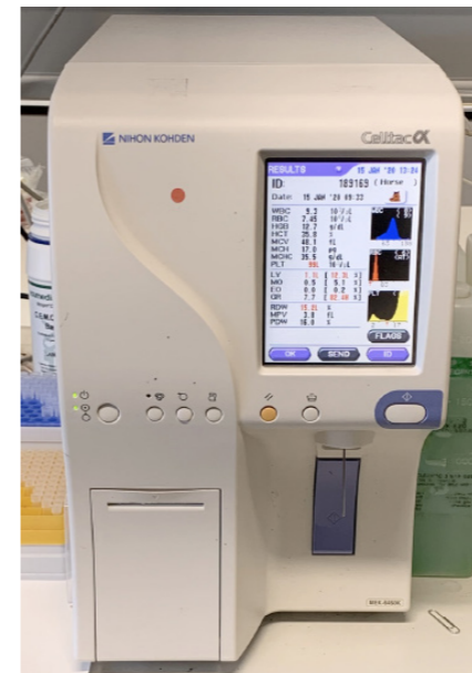
Figure 2 A haematology machine. This analyses the cells within blood, including red blood cells, white blood cells and platelets
